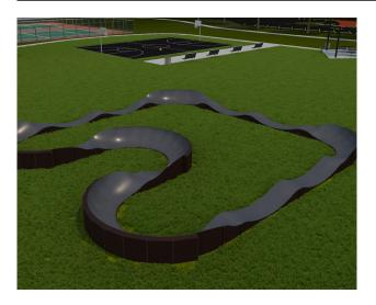
A Pumptrack is a progressive kind of structure that uses an up and down 'pumping' motion to propel the bicycle forward instead of pedaling.
